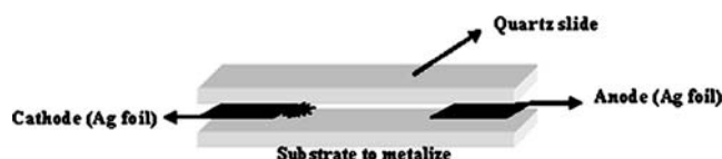
Scheme 1 Configuration for creation of fractal silver surfaces on silver electrodes and quartz glass
